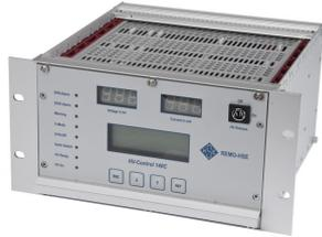
The control is equipped with a wide-range input with PFC, 4-line LCD-display and four membrane keys which makes it simple to operate, big 7-segment LED displays for current and volt-
